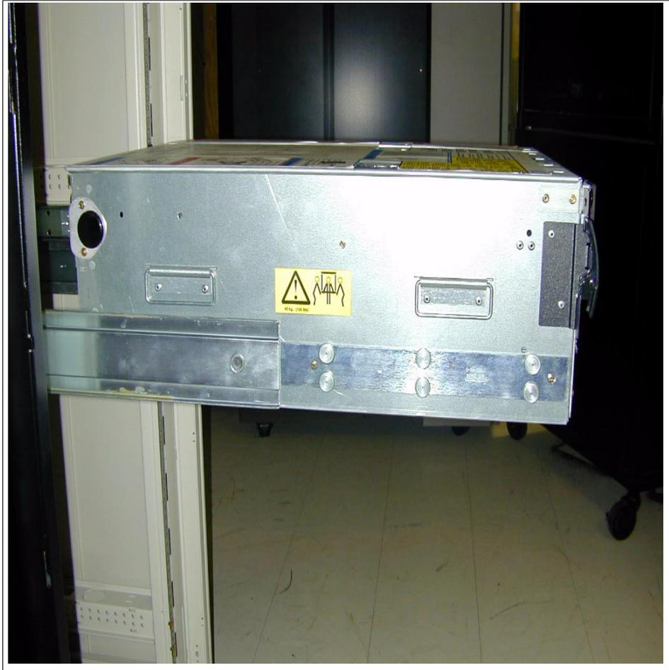
*Figure 3-19 System drawer in service position*
