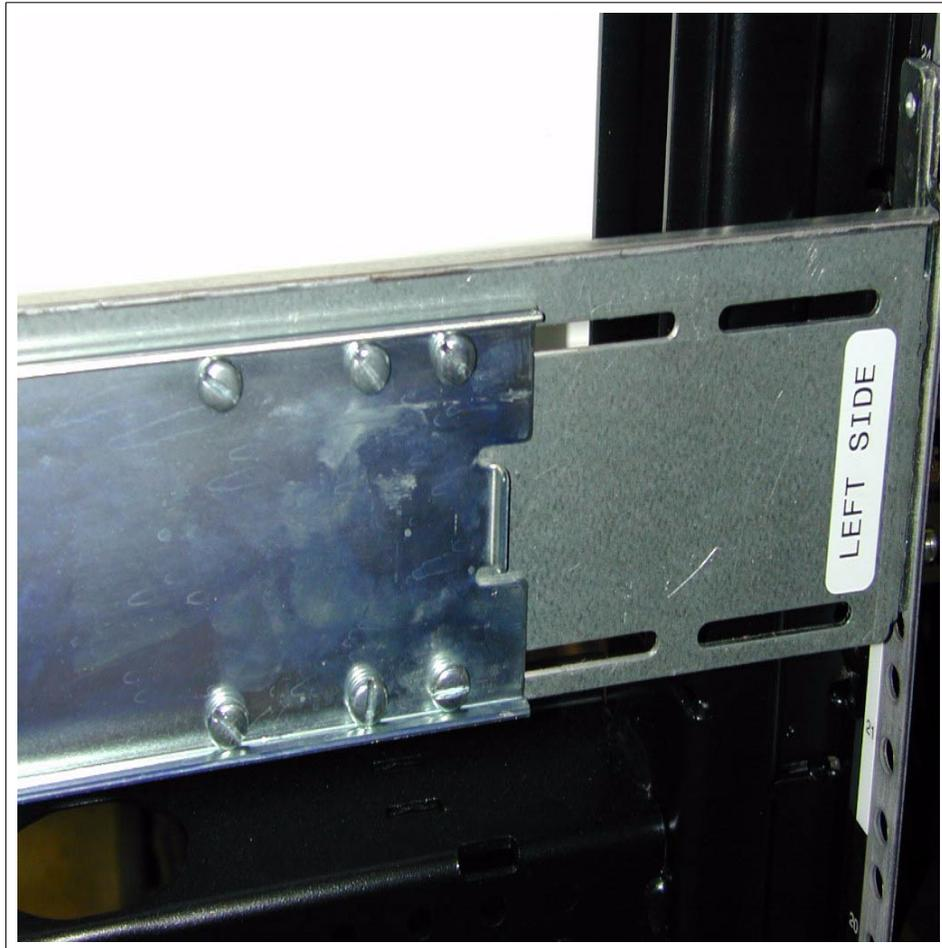
Figure 3-11 Rail length adjustment screws
