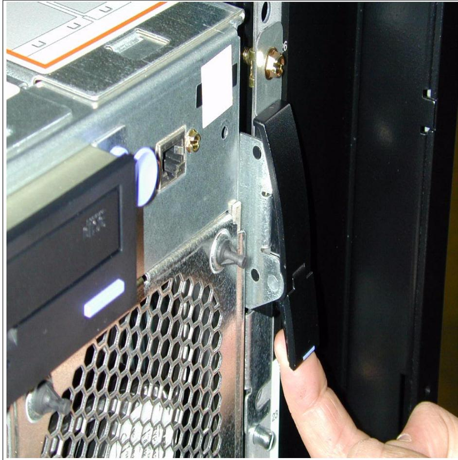
Figure 3-22 Lower section of release latch
